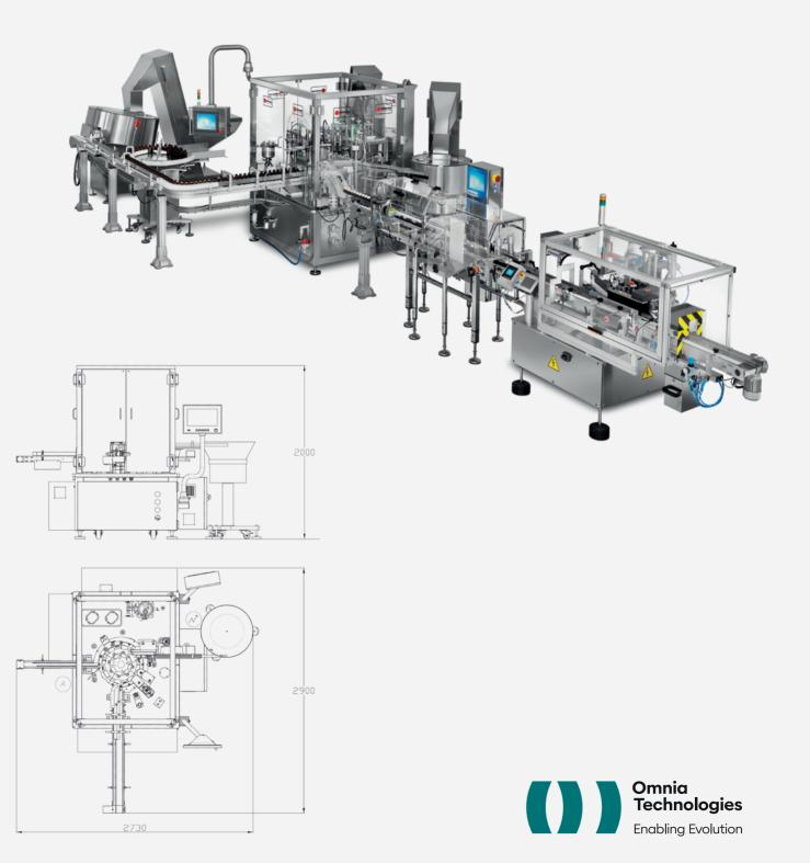
The **FD120** model is a versatile, indexing machine, designed to fill and close most pharmaceutical containers. Its robust design and traditional alternate motion ensures ideal flexibility and easy of use for both operators and maintenance technicians.
